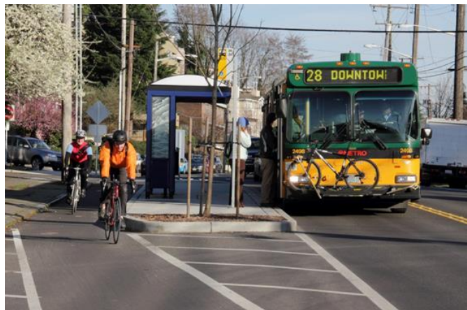
The bicycle lane was incorporated into the bus stop station design, allowing cyclists to safely pass the idling bus. Photo credit: City of Seattle.
