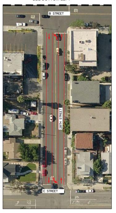
CONVERTING SEGMENTS OF 28TH STREET INTO 2 LANE COLLECTORS WITH CONTINUOUS LEFT—TURN LANES WOULD BE REQUIRED TO IMPROVE OPERATIONS OF THE ROADWAY SEGMENTS TO LOS D OR BETTER. AS SHOWN IN THE GRAPHIC, THESE ADDITIONAL LANES WOULD RESULT IN LOSS OF PARKING.
