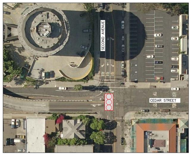
THE ADDITION OF A TRAFFIC SIGNAL WOULD BE REQUIRED TO IMPROVE OPERATIONS AT THE INTERSECTION OF CEDAR STREET AND SECOND AVENUE TO LOS D OR BETTER DURING BOTH PEAK HOURS.
