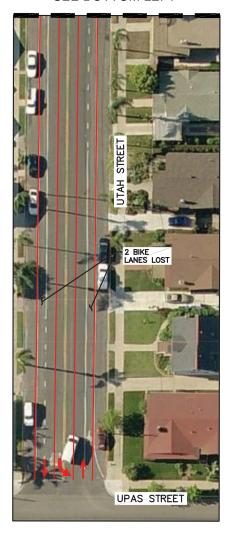
CONVERTING SEGMENTS OF UTAH STREET INTO 2 LANE COLLECTORS WITH CONTINUOUS LEFT—TURN LANES WOULD BE REQUIRED TO IMPROVE OPERATIONS OF THE ROADWAY SEGMENTS TO LOS D OR BETTER. AS SHOWN IN THE GRAPHIC, THESE ADDITIONAL LANES WOULD RESULT IN LOSS OF PARKING, AND IMPACT BICYCLE LANES.
