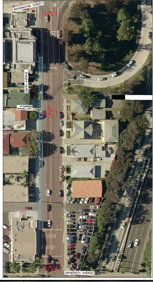
CONVERTING A SEGMENT OF NINTH AVENUE INTO A 2 LANE COLLECTOR WITH A CONTINUOUS LEFT TURN LANE WOULD BE REQUIRED TO IMPROVE OPERATIONS OF THE ROADWAY SEGMENT TO LOS D OR BETTER. AS SHOWN IN THE GRAPHIC, THIS ADDITIONAL LANE WOULD RESULT IN LOSS OF PARKING.
