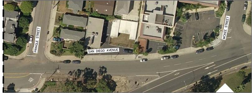
CONVERTING SEGMENTS OF SAN DIEGO AVENUE INTO 2 LANE COLLECTORS WITH CONTINUOUS LEFT—TURN LANES WOULD BE REQUIRED TO IMPROVE OPERATIONS OF THE ROADWAY SEGMENTS TO LOS D OR BETTER. AS SHOWN IN THE GRAPHIC, THESE ADDITIONAL LANES WOULD IMPACT BICYCLE LANES.
