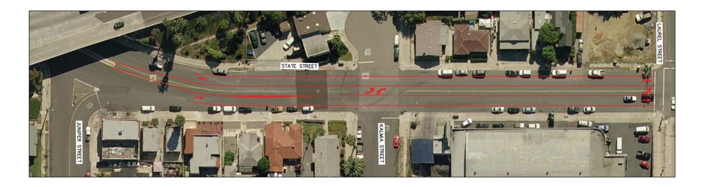
CONVERTING A SEGMENT OF STATE STREET INTO 2 LANE COLLECTOR WITH A CONTINUOUS LEFT—TURN LANE WOULD BE REQUIRED TO IMPROVE OPERATIONS OF THE ROADWAY SEGMENT TO LOS D OR BETTER. AS SHOWN IN THE GRAPHIC, THIS ADDITIONAL LANE WOULD CAUSE NO SIGNIFICANT IMPACTS TO EXISTING CONDITIONS.
