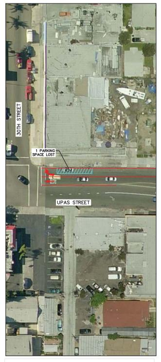
THE ADDITION OF A WESTBOUND LANE WOULD BE REQUIRED TO IMPROVE OPERATIONS AT THE INTERSECTION OF UPAS STREET AND 30TH STREET TO LOS D OR BETTER DURING BOTH THE AM AND PM PEAK HOURS. AS SHOWN IN THE GRAPHIC, THIS ADDITIONAL LANE WOULD RESULT IN LOSS OF PARKING.
