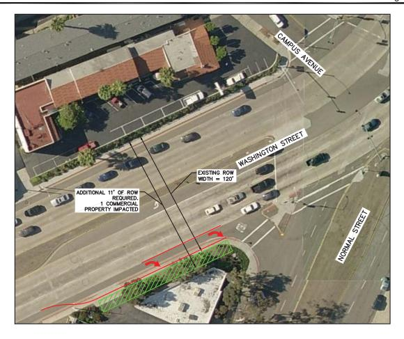
THE ADDITION OF A NORTH-EASTBOUND LANE WOULD BE REQUIRED TO IMPROVE OPERATIONS AT THE INTERSECTION OF WASHINGTON AVENUE, NORMAL STREET, CAMPUS AVENUE, AND POLK AVENUE TO LOS D OR BETTER DURING THE AM AND PM PEAK HOURS. AS SHOWN IN THE GRAPHIC, THIS ADDITIONAL LANE WOULD REQUIRE RIGHT-OF-WAY FROM ADJACENT PROPERTY.
