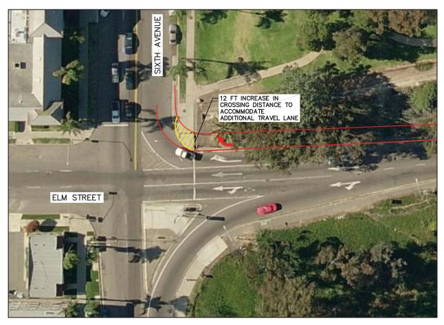
THE ADDITION OF A WESTBOUND LANE WOULD BE REQUIRED TO IMPROVE OPERATIONS AT THE INTERSECTION OF ELM STREET AND SIXTH AVENUE TO LOS D OR BETTER DURING THE AM PEAK HOUR. AS SHOWN IN THE GRAPHIC, THIS ADDITIONAL LANE WOULD INCREASE THE PEDESTRIAN CROSSING DISTANCE.
