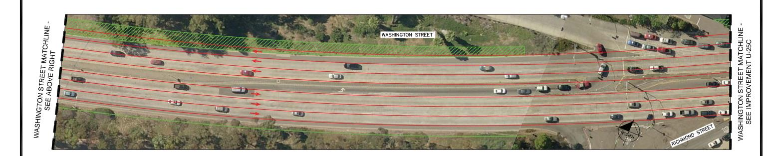
CONVERTING SEGMENTS OF WASHINGTON STREET INTO 6 LANE MAJOR ARTERIALS WOULD BE REQUIRED TO IMPROVE OPERATIONS OF THE ROADWAY SEGMENTS TO LOS D OR BETTER. AS SHOWN IN THE GRAPHIC, THESE ADDITIONAL LANES WOULD REQUIRE RIGHT-OF-WAY FROM ADJACENT PROPERTY AND BRIDGE WIDENING.
