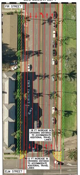
CONVERTING SEGMENTS OF SIXTH AVENUE INTO 4 LANE COLLECTORS WOULD BE REQUIRED TO IMPROVE OPERATIONS OF THE ROADWAY SEGMENTS TO LOS D OR BETTER. AS SHOWN IN THE GRAPHIC, THESE ADDITIONAL LANES WOULD REQUIRE RIGHT—OF—WAY FROM ADJACENT PROPERTY AND INCREASE THE PEDESTRIAN CROSSING DISTANCE.
