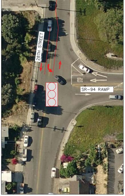
THE ADDITION OF A TRAFFIC SIGNAL AND A SOUTHBOUND LANE WOULD BE REQUIRED TO IMPROVE OPERATIONS AT THE INTERSECTION OF STATE ROUTE 94 EASTBOUND RAMPS AND 28TH STREET TO LOS D OR BETTER DURING BOTH THE AM AND PM PEAK HOURS. AS SHOWN IN THE GRAPHIC, THIS ADDITIONAL LANE WOULD CAUSE NO SIGNIFICANT IMPACTS TO EXISTING CONDITIONS
