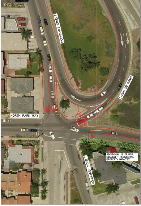
ADDITION OF A SECOND SOUTHBOUND LEFT TURN LANE AND AN EXCLUSIVE WESTBOUND LEFT TURN LANE WOULD BE REQUIRED TO IMPROVE OPERATIONS AT THE INTERSECTION OF NORTH PARK WAY AND I-805 SOUTHBOUND RAMPS TO LOS D OR BETTER DURING THE PM PEAK HOUR. AS SHOWN IN THE GRAPHIC, THESE IMPROVEMENTS WOULD REQUIRE RIGHT-OF-WAY FROM ADJACENT PROPERTY.
