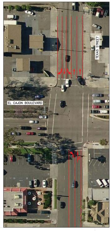
A RECONFIGURATION OF TEXAS STREET TO HAVE A NORTHBOUND LEFT AND SHARED THROUGH-RIGHT AND A SOUTHBOUND LEFT, ONE THROUGH, AND ONE RIGHT WOULD BE REQUIRED TO IMPROVE OPERATIONS AT THE INTERSECTION OF EL CAJON BOULEVARD AND TEXAS STREET TO LOS D OR BETTER DURING THE AM PEAK HOUR. AS SHOWN IN THE GRAPHIC, THIS RECONFIGURATION WOULD CAUSE NO SIGNIFICANT IMPACTS TO EXISTING CONDITIONS.
