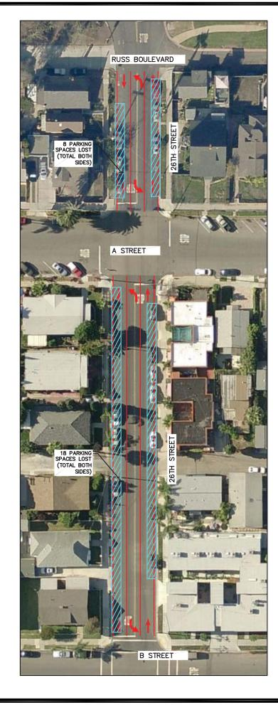
CONVERTING SEGMENTS OF 26TH STREET INTO 2 LANE COLLECTORS WITH CONTINUOUS LEFT—TURN LANES WOULD BE REQUIRED TO IMPROVE OPERATIONS OF THE ROADWAY SEGMENTS TO LOS D OR BETTER. AS SHOWN IN THE GRAPHIC, THESE ADDITIONAL LANES WOULD RESULT IN LOSS OF PARKING.
