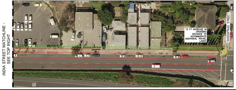
CONVERTING SEGMENTS OF INDIA STREET INTO 2 LANE COLLECTORS WITH CONTINUOUS LEFT TURN LANES, 3 LANE ONE—WAY COLLECTORS, AND 4 LANE ONE—WAY COLLECTORS WOULD BE REQUIRED TO IMPROVE OPERATIONS OF THE ROADWAY SEGMENTS TO LOS D OR BETTER. AS SHOWN IN THE GRAPHIC, THESE ADDITIONAL LANES WOULD REQUIRE RIGHT—OF—WAY FROM ADJACENT PROPERTY, INCREASE PEDESTRIAN CROSSING DISTANCE, AND RESULT IN LOSS OF PARKING.
