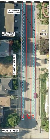
CONVERTING SEGMENTS OF FLORIDA STREET INTO 2 LANE COLLECTORS WITH A CONTINUOUS LEFT—TURN LANE WOULD BE REQUIRED TO IMPROVE OPERATIONS OF THE ROADWAY SEGMENTS TO LOS D OR BETTER. AS SHOWN IN THE GRAPHIC, THIS ADDITIONAL LANE WOULD RESULT IN LOSS OF PARKING.
