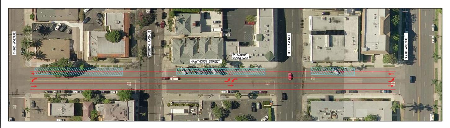
CONVERTING A SEGMENT OF HAWTHORN STREET INTO A 2 LANE COLLECTOR WITH A CONTINUOUS LEFT TURN LANE WOULD BE REQUIRED TO IMPROVE OPERATIONS OF THE ROADWAY SEGMENT TO LOS D OR BETTER. AS SHOWN IN THE GRAPHIC, THIS ADDITIONAL LANE WOULD RESULT IN LOSS OF PARKING.
