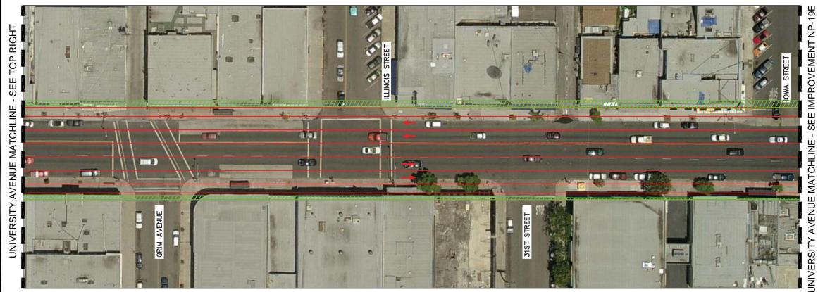
CONVERTING SEGMENTS OF UNIVERSITY AVENUE INTO 4 LANE COLLECTORS WOULD BE REQUIRED TO IMPROVE OPERATIONS OF THE ROADWAY SEGMENTS TO LOS D OR BETTER. AS SHOWN IN THE GRAPHIC, THESE ADDITIONAL LANES WOULD REQUIRE RIGHT—OF—WAY FROM ADJACENT PROPERTY AND INCREASE PEDESTRIAN CROSSING DISTANCES.
