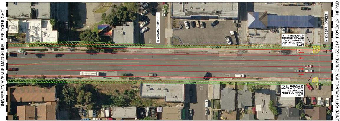
CONVERTING SEGMENTS OF UNIVERSITY AVENUE INTO 4 LANE COLLECTORS WOULD BE REQUIRED TO IMPROVE OPERATIONS OF THE ROADWAY SEGMENTS TO LOS D OR BETTER. AS SHOWN IN THE GRAPHIC, THESE ADDITIONAL LANES WOULD REQUIRE TUNNEL WIDENING AND INCREASE PEDESTRIAN CROSSING DISTANCES.
