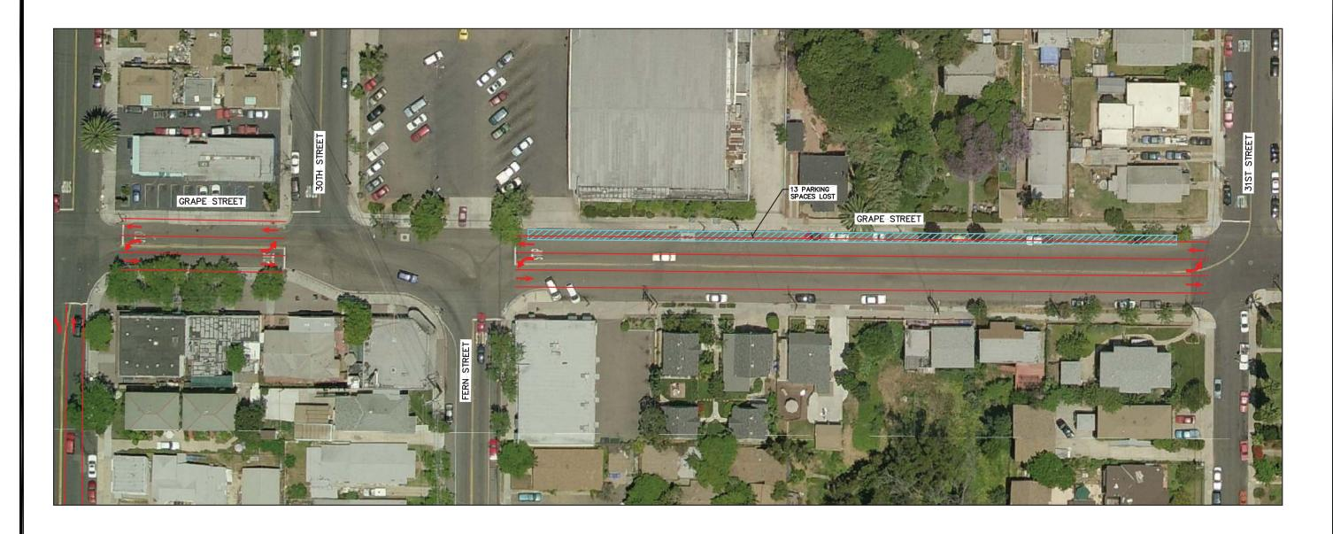
CONVERTING A SEGMENT OF GRAPE STREET INTO A TWO LANE COLLECTOR WITH A CONTINUOUS LEFT—TURN LANE WOULD BE REQUIRED TO IMPROVE OPERATIONS OF THE ROADWAY SEGMENTS TO LOS D OR BETTER. AS SHOWN IN THE GRAPHIC, THIS ADDITIONAL LANE WOULD RESULT IN LOSS OF PARKING.
