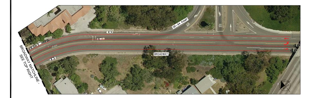
CONVERTING A SEGMENT OF BROADWAY INTO A 2 LANE COLLECTOR WITH A CONTINUOUS LEFT—TURN LANE WOULD BE REQUIRED TO IMPROVE OPERATIONS OF THE ROADWAY SEGMENT TO LOS D OR BETTER. AS SHOWN IN THE GRAPHIC, THESE CHANGES WOULD NOT HAVE A SIGNIFICANT IMPACT ON EXISTING CONDITIONS.
