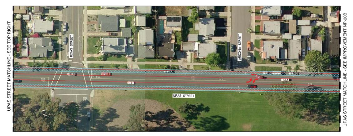
CONVERTING SEGMENTS OF UPAS STREET INTO A 2 LANE COLLECTOR WITH A CONTINUOUS LEFT—TURN LANE WOULD BE REQUIRED TO IMPROVE OPERATIONS OF THE ROADWAY SEGMENTS TO LOS D OR BETTER. AS SHOWN IN THE GRAPHIC, THIS ADDITIONAL LANE WOULD RESULT IN LOSS OF PARKING.
