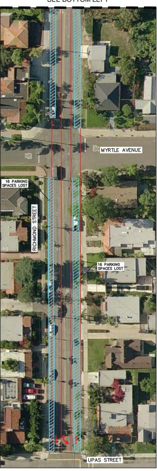
CONVERTING SEGMENTS OF RICHMOND STREET INTO 2 LANE COLLECTORS WITH CONTINUOUS LEFT—TURN LANES WOULD BE REQUIRED TO IMPROVE OPERATIONS OF THE ROADWAY SEGMENTS TO LOS D OR BETTER. AS SHOWN IN THE GRAPHIC, THESE ADDITIONAL LANES WILL RESULT IN LOSS OF PARKING.
