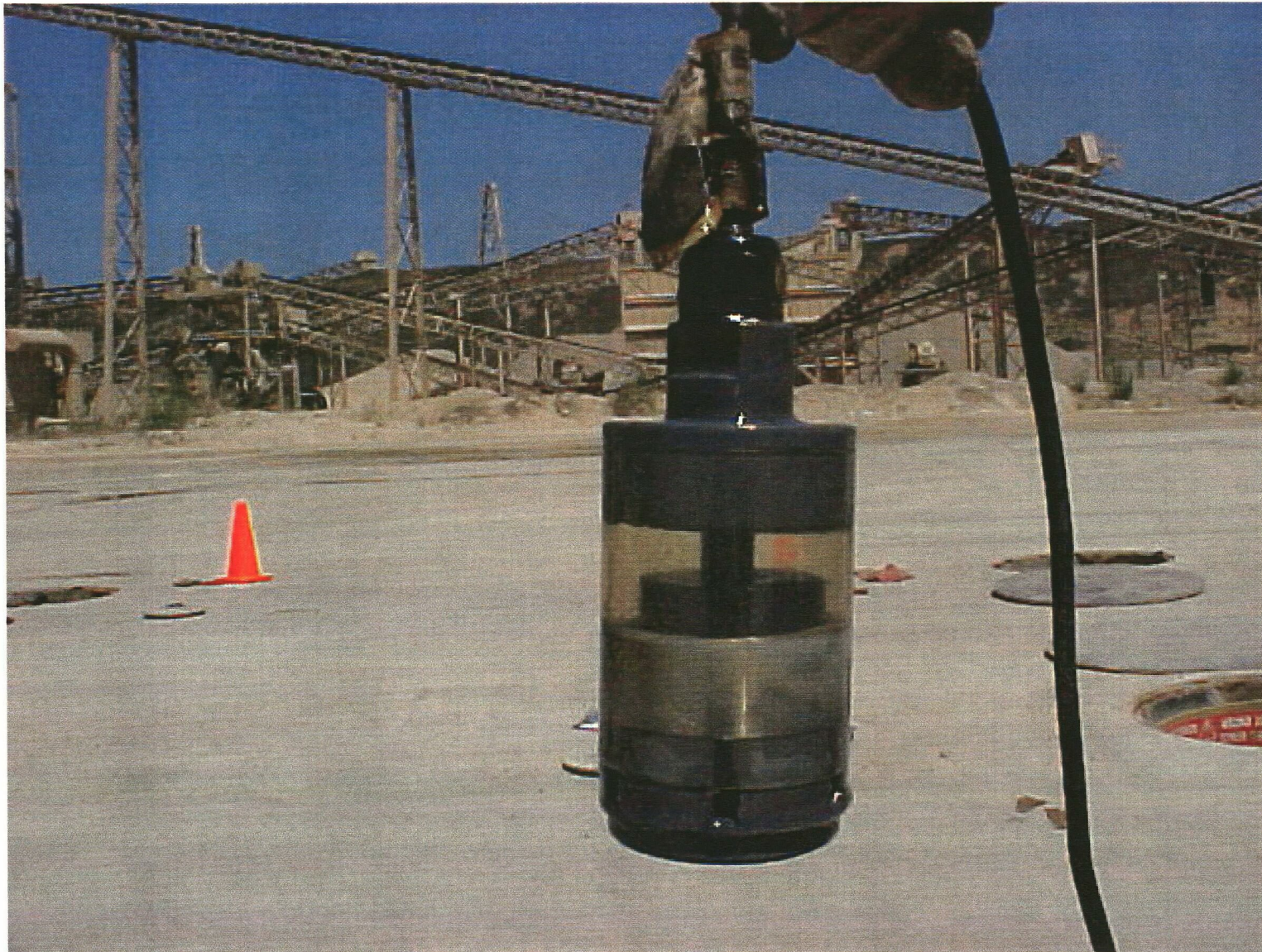
Brine filled annular space sensors are the “single-float” variety; they are only capable of detecting low brine levels.
