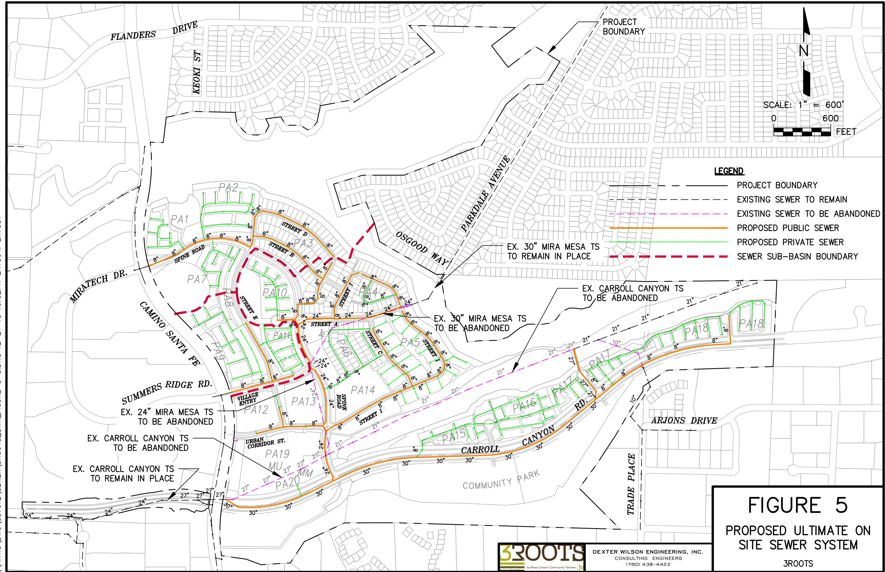
**Onsite Private Sewer System Slopes.** Many of the Planning Areas are proposed to have private onsite sewer systems. These systems will be designed to maintain a minimum of one (1) percent slope to meet plumbing code standards. Alternatively, the private sewer systems within the Planning Areas may be designed in accordance with the City of San Diego Sewer Design Guide.
