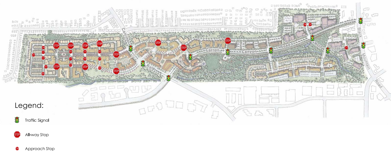
Figure 6-5. Stone Creek Intersection and Traffic Control Plan
