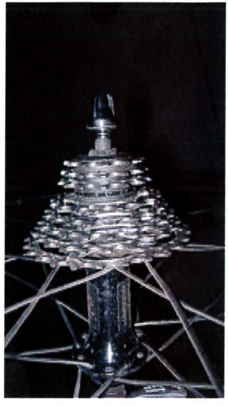
Rear cassette is numbered from low gear to high gear. Each sprocket is a gear.
