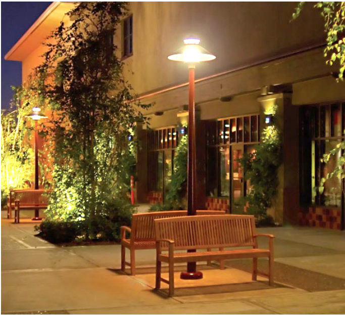
Lighting should be directed downward onto the sidewalk with fully shielded fixtures.
