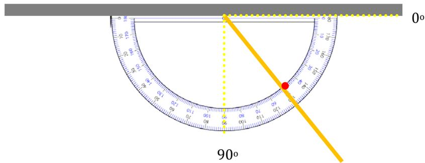
The angle between the surface and the probe can be measured. In this example, the angle is 51 degrees. The bullet can then be reported as traveling right to left at an angle of 51 degrees. If you want to report the angle from the shooter's perspective (NATO method), use the complementary angle ( $90 - 51$ ). Then the angle would be reported as "the shooter fired the gun from 39 degrees right of perpendicular."
