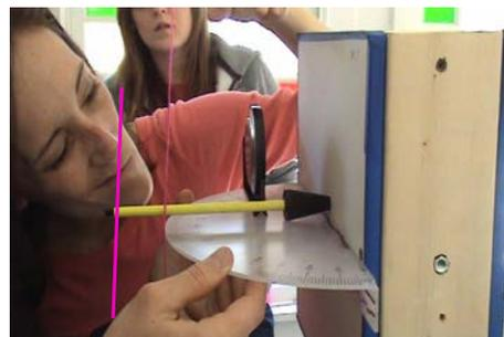
1. Press the protractor up against the surface of the impact. This can be a wall, a windshield, a chair, or any other flat surface that is impacted by the bullet.
