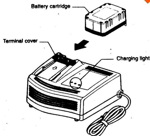
1. Insert the battery cartridge into the charger until it stops adjusting to the guide of the charger. The terminal cover of the charger can be opened with inserting and closed with pulling out the battery cartridge.
