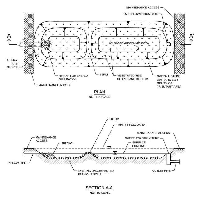
Figure E.9-E.9-1: Typical plan and section view of an Infiltration BMP
