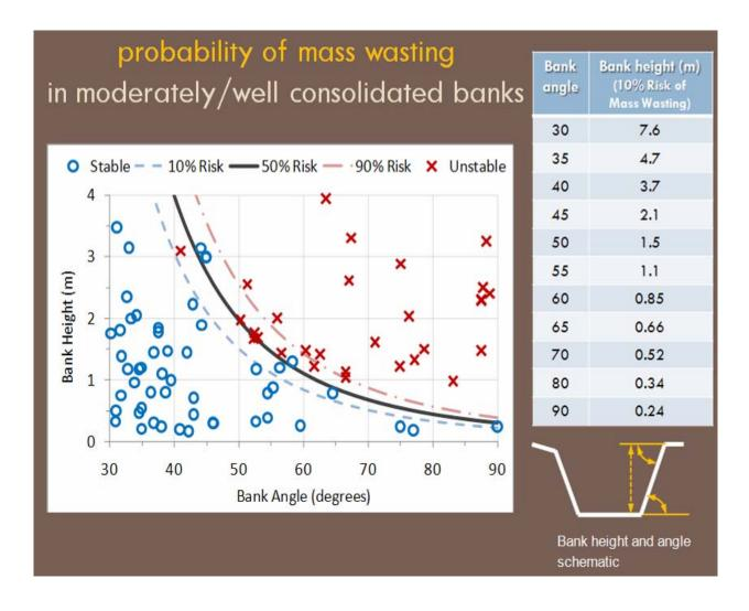
Form 6 Figure 1. Probability Mass Wasting diagram, Bank Angle:Height/% Risk table, and Band Height:Angle schematic.
