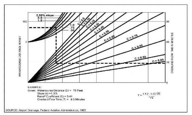
Figure A-4. Rational Formula - Overland Time of Flow Nomograph
