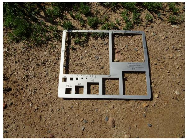
Figure 14. Gravelometer Reflecting Typical Material in Study Reaches
