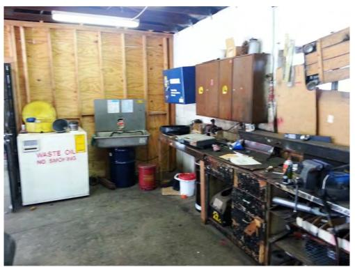
**Photo 13**: View inside the maintenance building in the central portion of the Site. A 130 gallon waste oil AST and parts washer are visible in the photograph.
