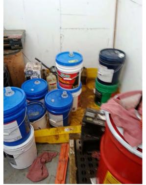
**Photo 14**: View of secondary containment for oil storage in the maintenance area in the central portion of the Site.
