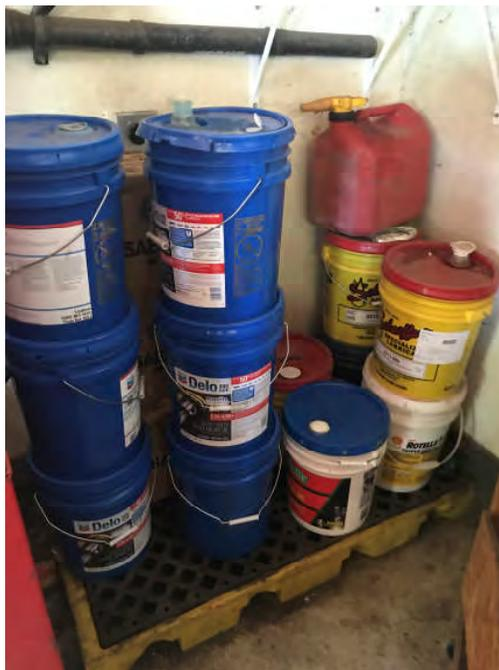
**Photo #34** View of 5-gallon buckets of lubricants, oils, and greases. These containers are stored on a secondary containment unit.
