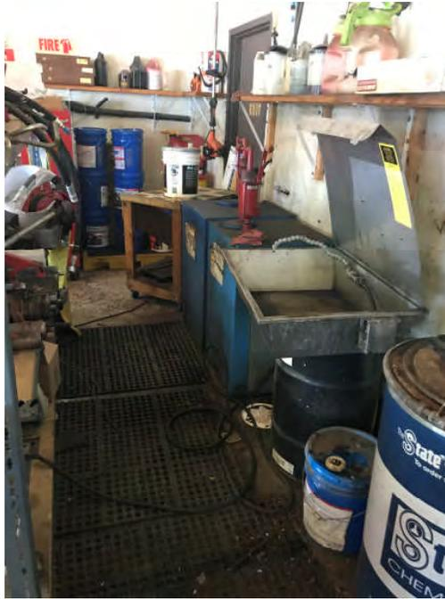
**Photo #33** View of 100-gallon tractor hydraulic fluid AST, 100-gallon new oil AST, animal-based solvent wash station with sink, and 55-gallon drum of granular absorbent. No secondary containment was observed for these features.
