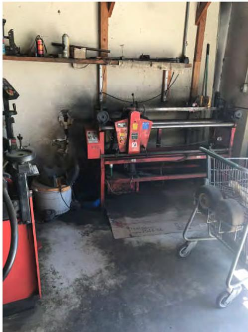
**Photo #28** View of a machinist lathe located in the maintenance shop. Flooring located beneath the lathe was observed to be heavily stained with gear lubricant.
