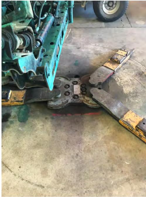
**Photo #31** View of a single-post in-ground hydraulic lift centrally located within the maintenance building. Surface staining was visible around the piston of the lift.
