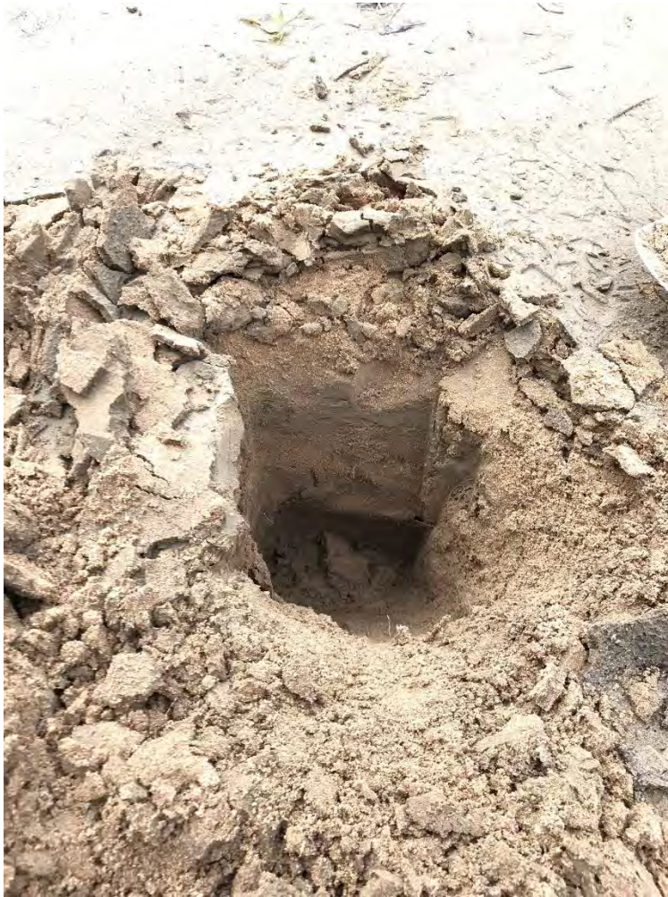
Photo 1.32: Soil Pit 1 in the detention basin showing deposition layers of sand and sandy loam.
