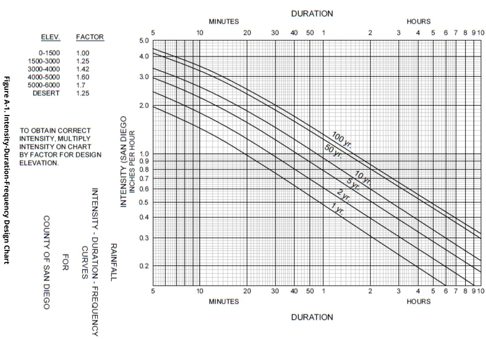
**Figure A-1. Intensity-Duration-Frequency Design Chart**
