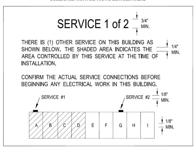
The plaque or directory required by Section 230.2(E) shall be manufactured in metal or plastic, suitable for the environment, with engraved or machine-printed lettering or electro-photo-plating in a contrasting color. The plaque shall include a properly orientated footprint of the entire building, with the area served by each service clearly delineated. The plaques shall be located at the service disconnect and securely fastened by permanent means acceptable to the AHJ.
