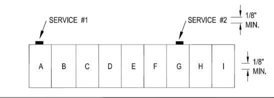
The plaque or directory shall be manufactured in metal or plastic, suitable for the environment, with engraved or machine-printed lettering or electro-photo-plating in a contrasting color. The plaque shall include a properly oriented footprint of the entire building. The plaques shall be located at the service disconnect and securely fastened by permanent means acceptable to the AHJ.
