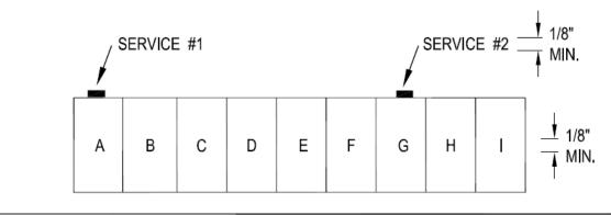
The plaque or directory shall be manufactured in metal or plastic, suitable for the environment, with engraved or machine-printed lettering or electro-photo-plating in a contrasting color. The plaque shall include a properly oriented footprint of the entire building, properly oriented, with the area served by each service clearly delineated. The plaques shall be located at the service disconnect and securely fastened by permanent means acceptable to the AHJ.
