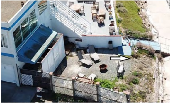
Augmented upper bluff on Nrth End. Bluff Edge on prior Geotechnical Report defined by gravel.
