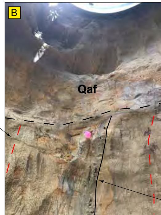
B) Looking upward towards contact between Artificial Fill materials and Damage Zone.
