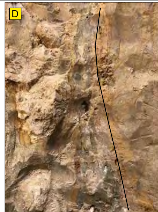
C - E) Close up of the Principal Slip Surface and aligned gravels in the Damage Zone.
