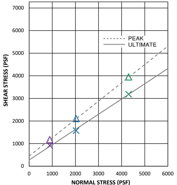
**DIRECT SHEAR - ASTM D 3080**
