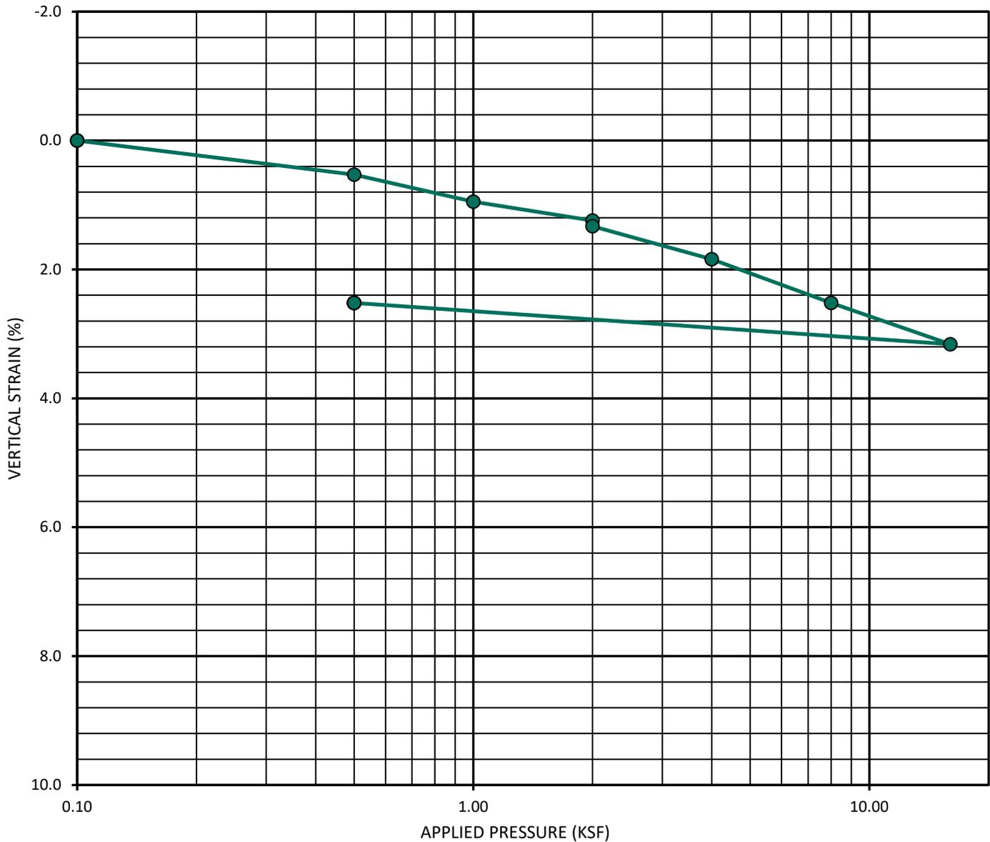
**CONSOLIDATION CURVE - ASTM D 2435**
