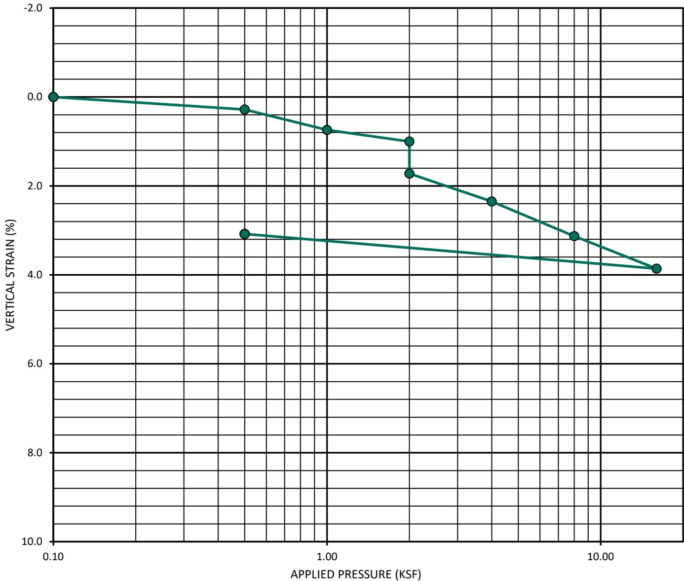
**CONSOLIDATION CURVE - ASTM D 2435**
