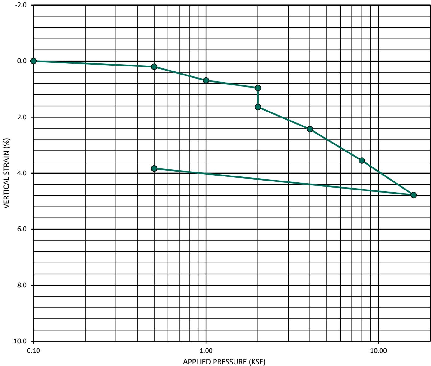
**CONSOLIDATION CURVE - ASTM D 2435**
