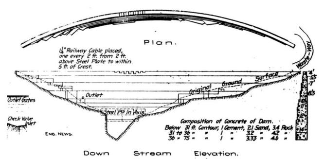
CORE FIG. 10. PLAN, ELEVATION AND DETAIL OF UPPER OTAY CONCRETE DAM, WITH STEEL PLATES AND CABLES, AS INDICATED.
