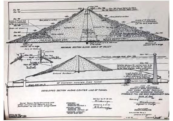
Figure 16. Combination Dam Design by H.N. Savage, approved 1932. (Hiram N. Savage Papers Collection, 1905-1933, Water Resources Collections and Archives, University of California, Riverside).
