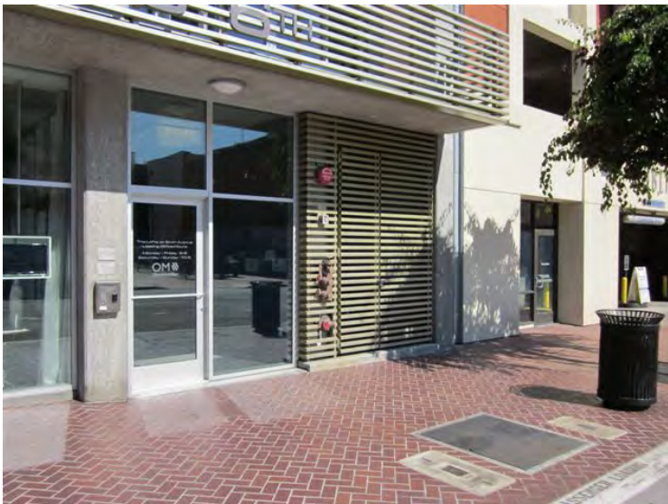
Backflow-prevention devices are to be located in a building alcove, landscaped area, or utility room within the building, outside of the public right-of-way, and completely screened from view. Above, San Diego, CA.
