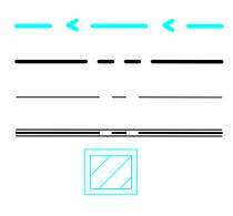
FLOW DIRECTION PROPERTY LINE ROAD CENTERLINE STORM DRAIN PIPE PUBLIC STORM DRAIN INLET
