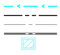
FLOW DIRECTION PROPERTY LINE ROAD CENTERLINE STORM DRAIN PIPE PUBLIC STORM DRAIN INLET
