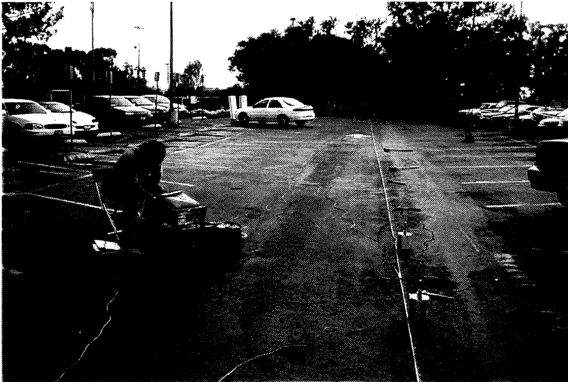
Figure 3 SASW Testing with Various Hammers as the Seismic Source.
