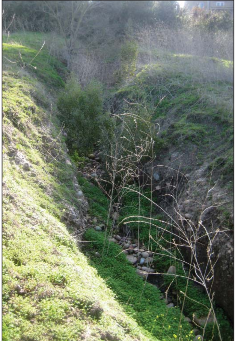
PHOTOGRAPH 1 View of Single-thread Channel Form with OHWM Indicators Low-flow Channel with Distinct Bed and Bank and Slumping Banks
