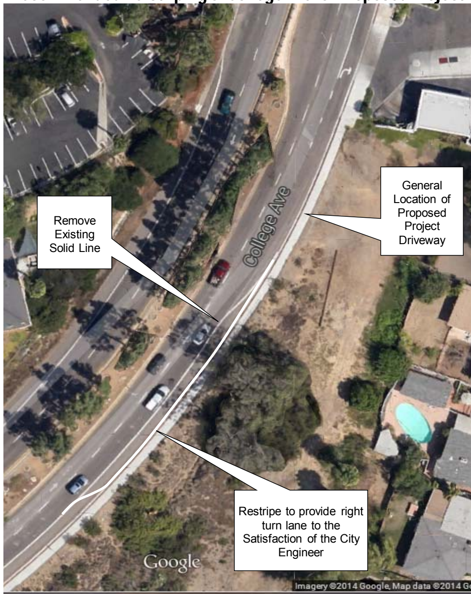
Figure 11: Recommended Re-Striping of College Ave for Proposed Project Driveway
