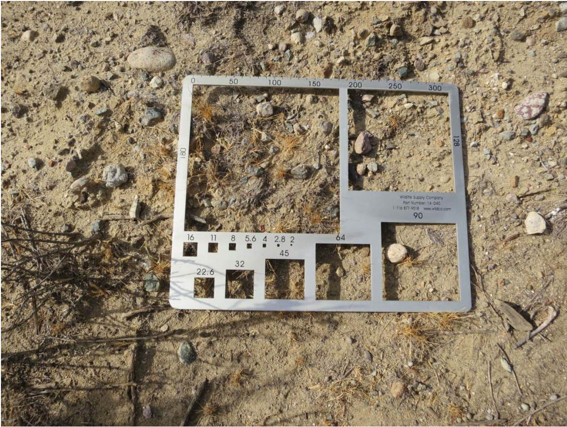
Figure 9. Gravelometer in Reach 1
