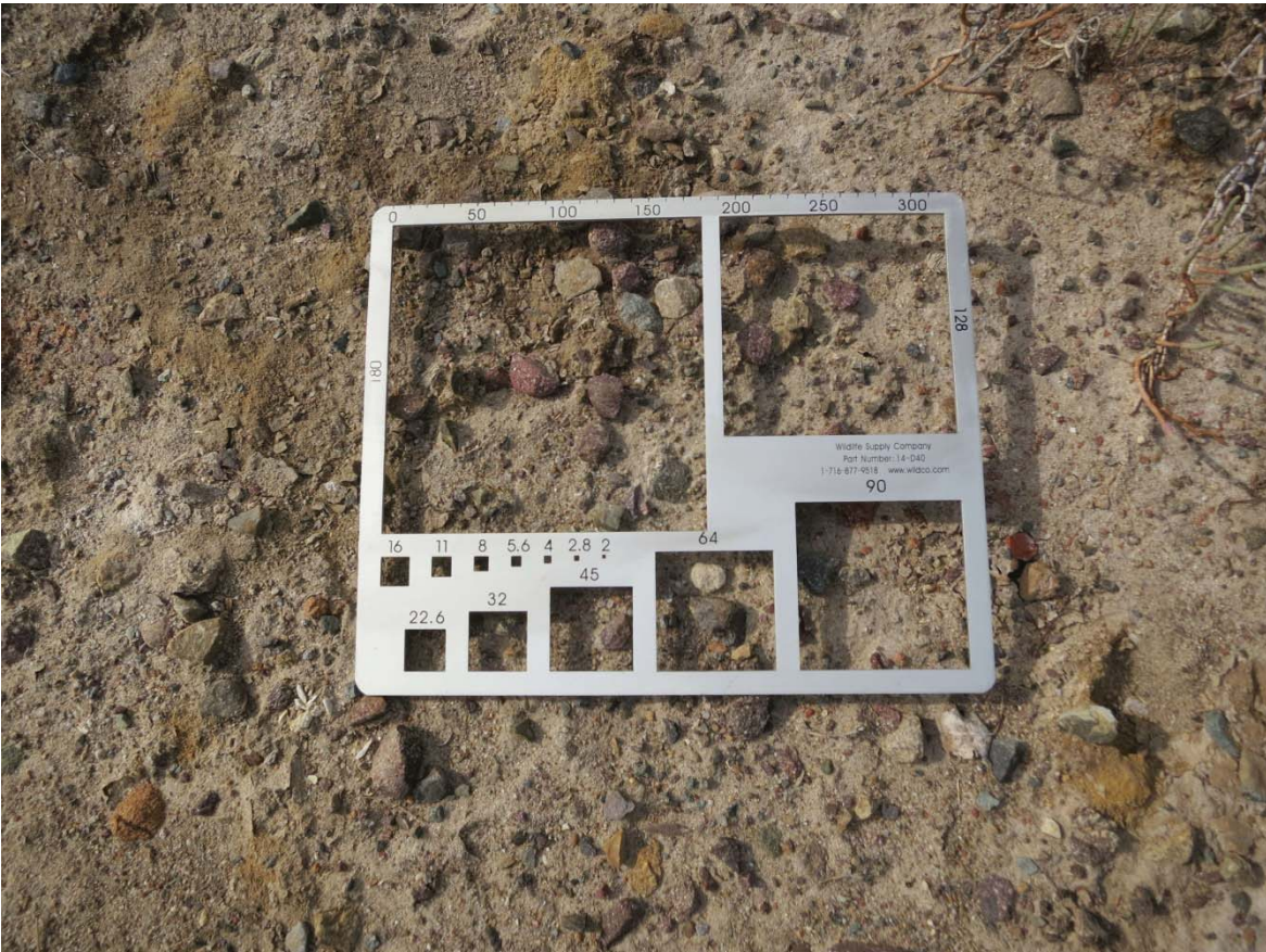
Figure 10. Gravelometer in Reach 2
