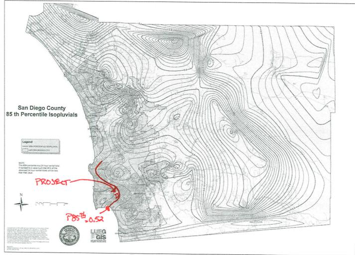
Figure B.1-1: 85th Percentile 24-hour Isopluvial Map
