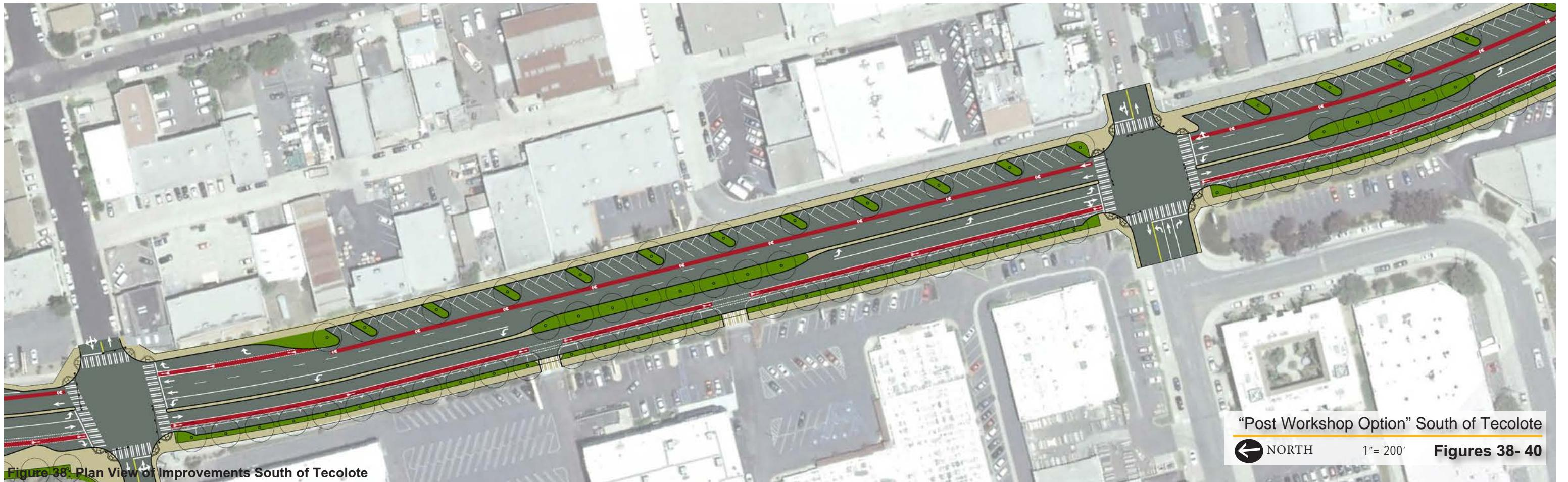
**Figure 39: One Lane Southbound with Green Backed Sharrows Lane Northbound**    **Section 1: Clairemont Trolley Station**
