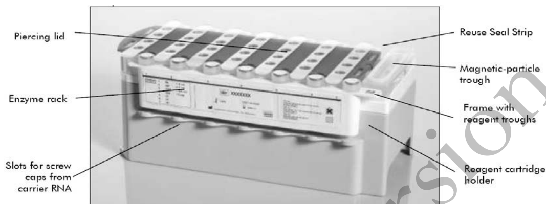
FIGURE 2 – ASSEMBLED COMPONENTS OF THE REAGENT CARTRIDGE
