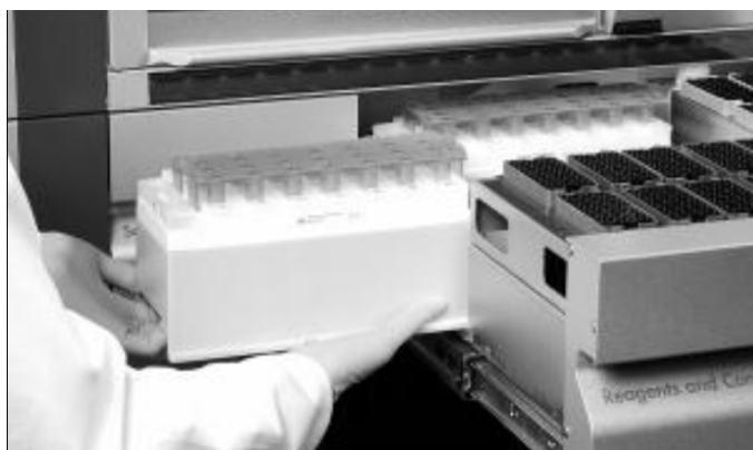
FIGURE 4 – SLIDING IN THE REAGENT CARTRIDGE
