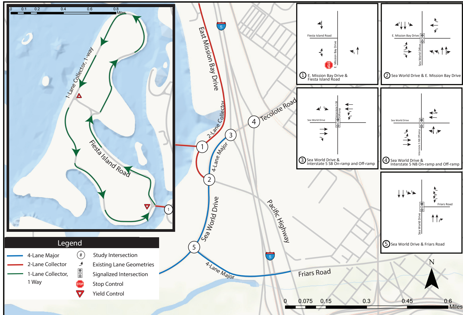
Figure 2-16 Existing Intersection Geometry and Functional Classifications
