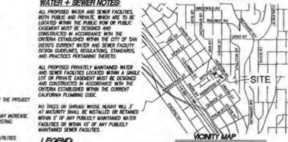
WATER + SEWER NOTES: ALL PROPOSED WATER AND SEWER FACILITIES, BOTH PUBLIC AND PRIVATE, WHICH ARE TO BE LOCATED WITHIN THE PUBLIC ROW OR PUBLIC EASEMENT MUST BE DESIGNED AND CONSTRUCTED IN ACCORDANCE WITH THE CRITERIA ESTABLISHED WITHIN THE CITY OF SAN DIEGO'S CURRENT WATER AND SEWER FACILITY DESIGN GUIDELINES, REGULATIONS, STANDARDS, AND PRACTICES PERTAINING THERETO.
