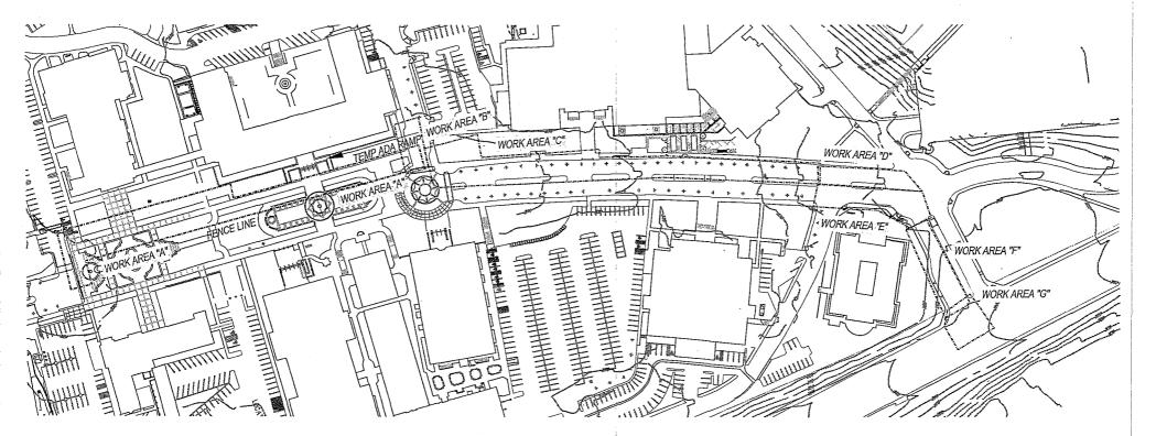
The fence line location is for illustration. During construction, the fence location and alignment will be finalized by coordinating with University of San Diego Campus Staff through the assigned Resident Engineer. The fence will also be located where it is applicable during the new water mains installation, in addition to the services installation where it is needed, and all associated work, and until completion of the project.
