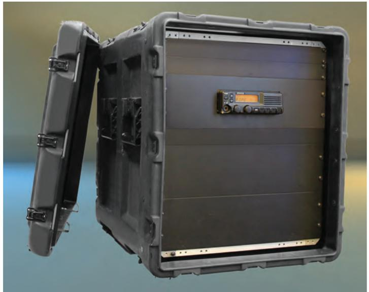
The US Digital Designs Portable Station Controller includes an ATX Station Controller, AC UPS, 12 Volt Radio Power Supply and Radio Mounting Panel in a ruggedized transport case with internal vibration-isolated rack frame.
