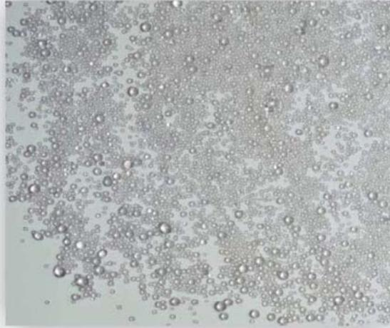
Quality glass beads that provide good, consistent retroreflective values in all conventional road marking materials. Used for inter-mix or drop-on applications and produced to meet all federal, state, county, or customer specifications.
