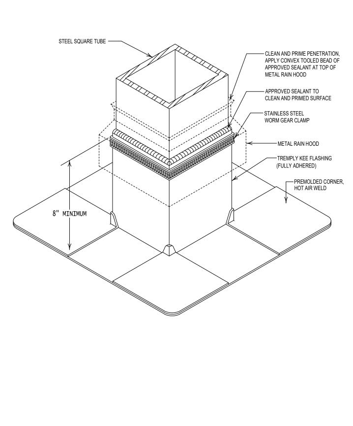
TREMPLY KEE FIELD FABRICATED SQUARE TUBE FLASHING **DWG NO. 20**
