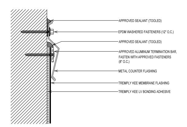
TREMPLY KEE WALL FLASHING TERMINATION'S DWG NO. 07
