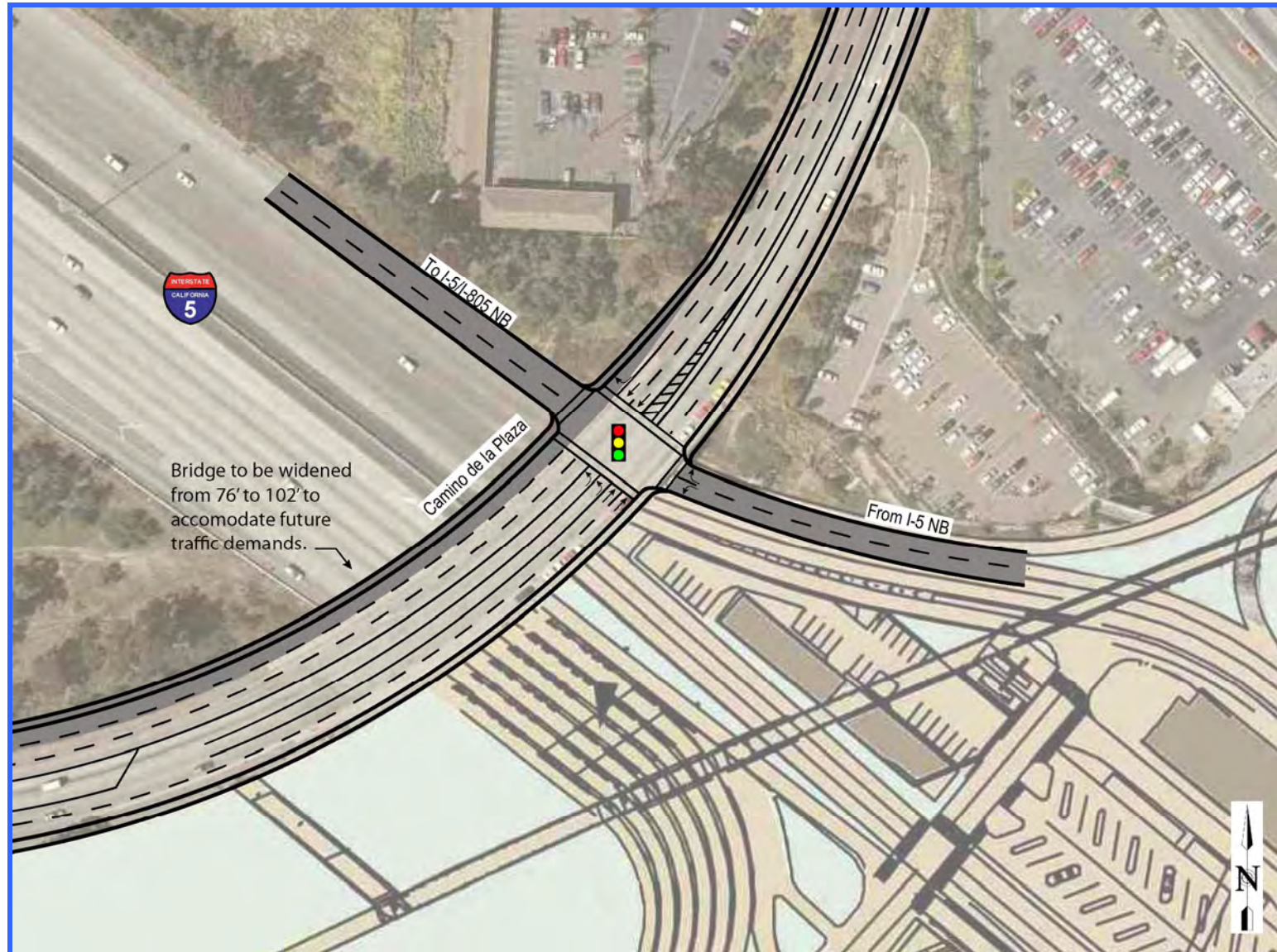
FIGURE 29: CONCEPTUAL LAYOUT OF PROPOSED CAMINO DE LA PLAZA/I-5 NORTHBOUND RAMPS
