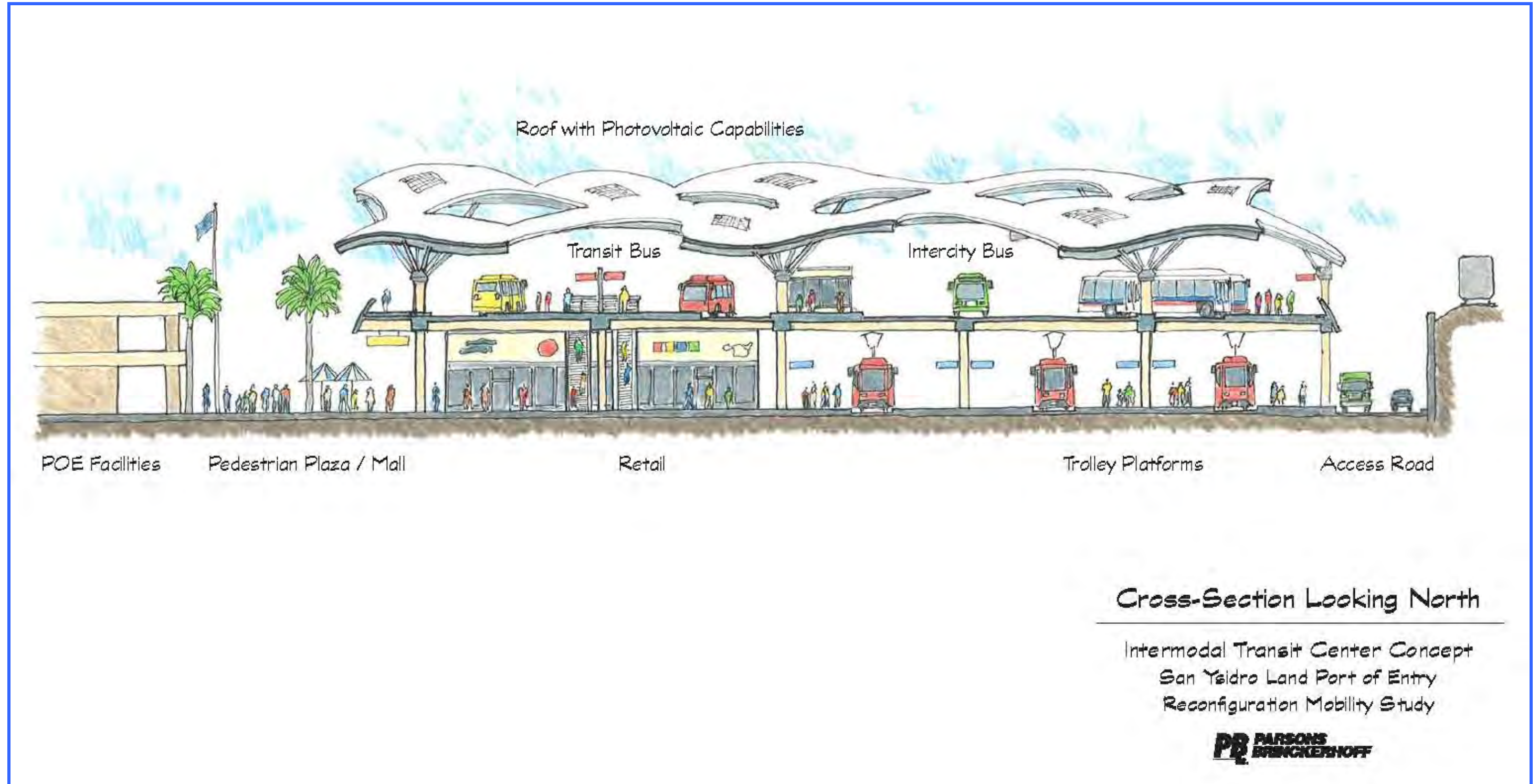
FIGURE 28: PREFERRED CONCEPT SITE DESIGN CROSS SECTION AT TRANSIT FACILITY (LOOKING NORTH)
