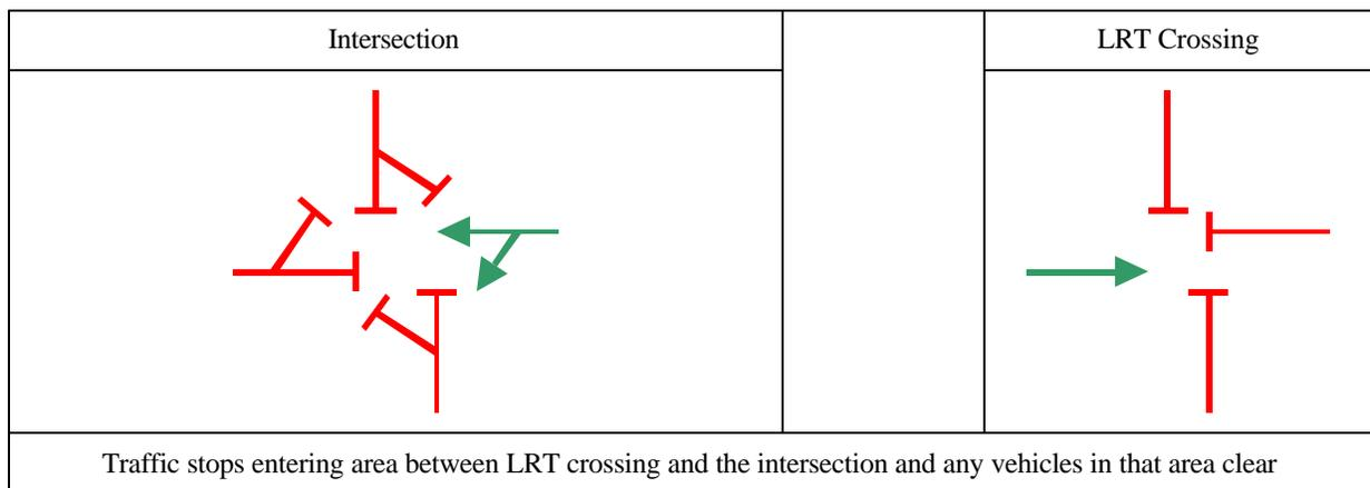
**Figure 3: Sequence of Controller Operation, LRT Approaching**
