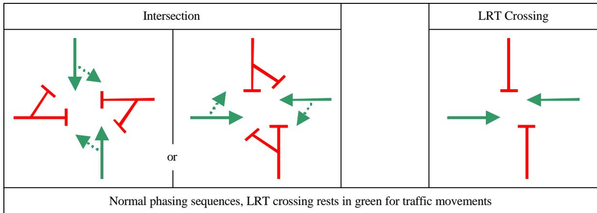
**Figure 2: Sequence of Controller Operation, No LRT**
