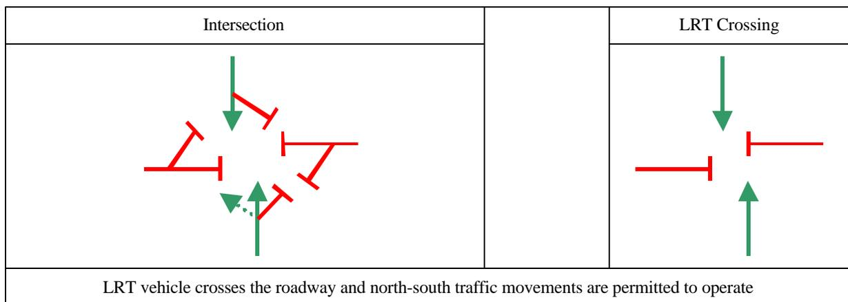
**Figure 4: Sequence of Controller Operation, LRT Crossing**
