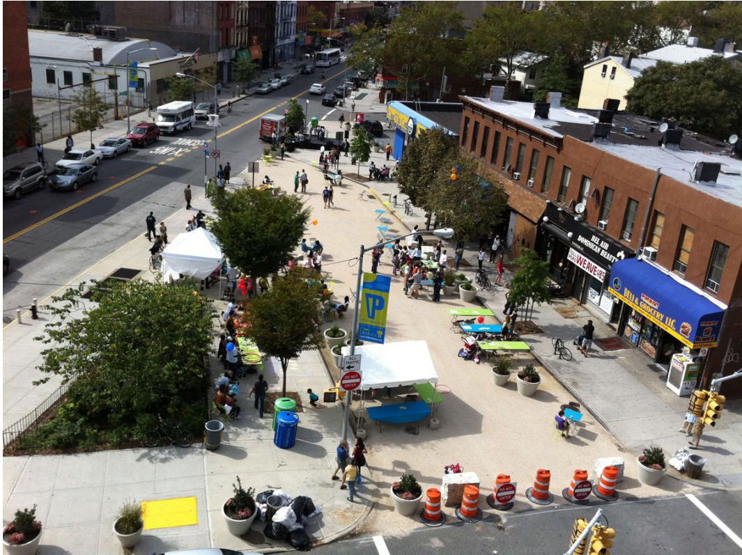
Figure 21 Use Re-stripping to Create Curb Extensions, Public Space
