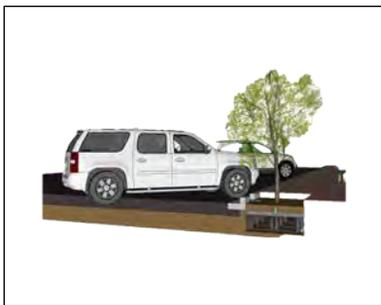
Image above highlights the use of Silva cells with tree grates and expanded sidewalk
