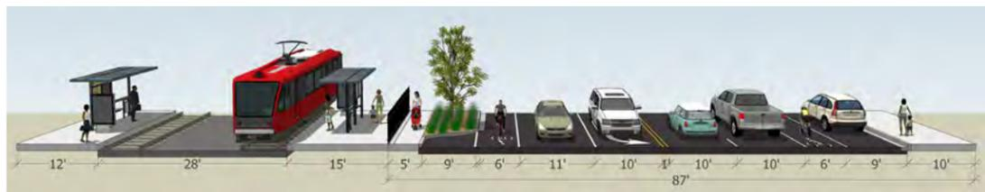
Figure ES-8: Cross Section 1: Clairemont LRT Station Area Improvements
