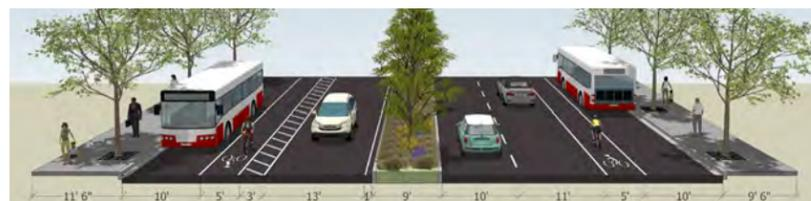
Figure ES-11: Cross Section 4: Tecolote LRT Station Area Improvements
