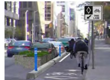
Figure 39: Raised Curb with Candlestick Markers on Curb
