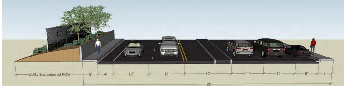
**Figure 22** Section 2: Existing Cross Section South of Ingulf
