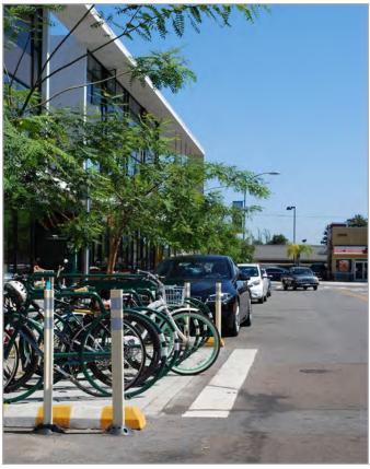
Bike corrals can accommodate more bicycle parking than typical sidewalk bicycle racks, especially where sidewalk widths are limited in width.
