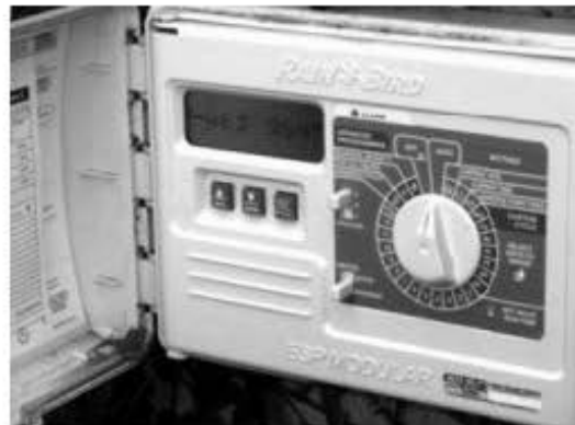
Weather Based Irrigation Controller made by Rain Bird - a leading manufacturer for home-based and professional irrigation systems.
