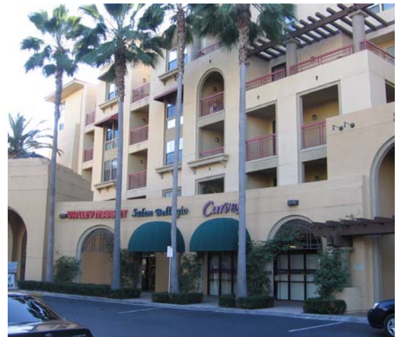
Awnings, trellises, and arcades can be used to identify and accentuate commercial uses on the ground level
