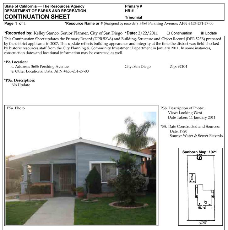
\*B6. Construction History: (Construction date, alterations, and date of alterations) A large addition has been constructed to the north of the porch. The porch has been partially enclosed with cement block. Brickwork at the porch has been painted. Windows have been replaced in original and altered openings. The original scored concrete walkway has been replaced.
