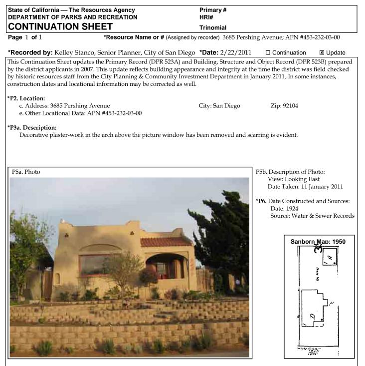
\*B6. Construction History: (Construction date, alterations, and date of alterations) Decorative plaster-work in the arch above the picture window has been removed and scarring is evident. Extensive retaining walls have been constructed in the front yard.
