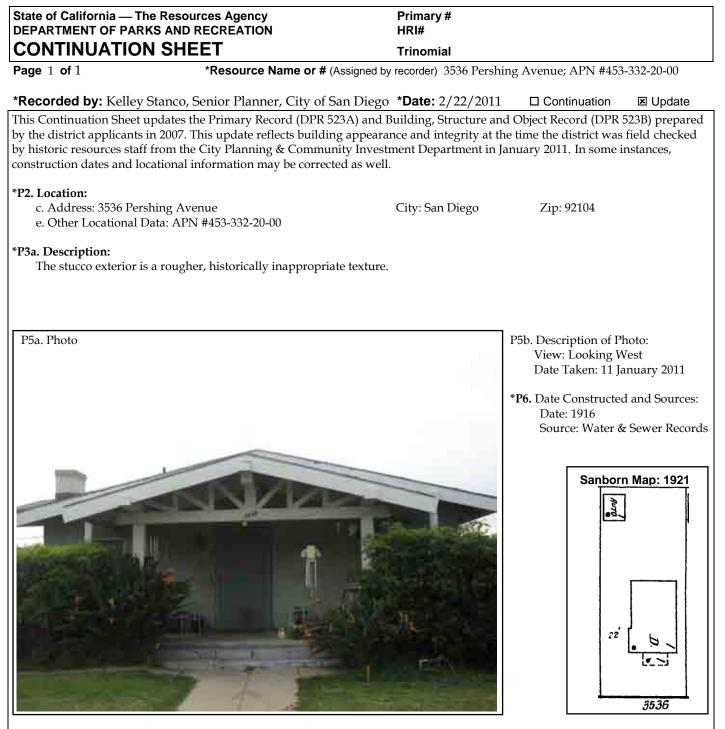
\*B6. Construction History: (Construction date, alterations, and date of alterations) The stucco exterior is a rougher, historically inappropriate texture. The original windows have been replaced with aluminum frame and sash windows. It is unknown whether this occurred in the original or altered openings.
