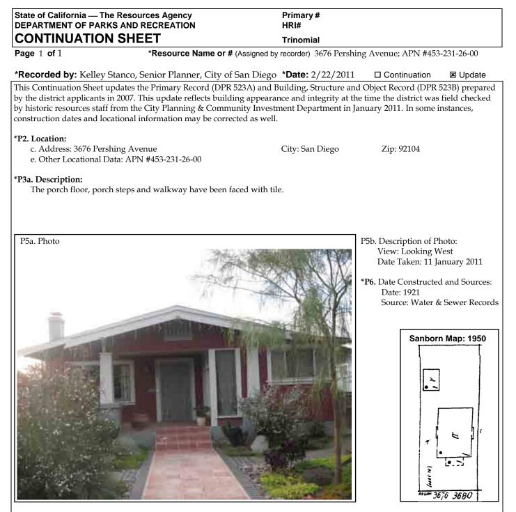
\*B6. Construction History: (Construction date, alterations, and date of alterations) The north end of the porch has been enclosed and an addition was constructed to the north of the porch. The windows have been replaced in new openings. The porch floor, porch steps and walkway have been faced with tile.
