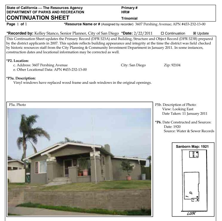
\*B6. Construction History: (Construction date, alterations, and date of alterations) An addition has been constructed at the south side of the house toward the rear. Vinyl windows have replaced wood frame and sash windows in the original openings.
