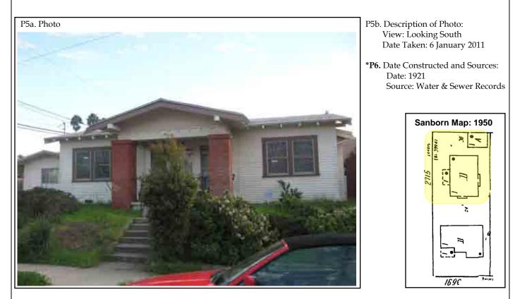
\*B6. Construction History: (Construction date, alterations, and date of alterations) The massive brick piers at the porch may be a later modification. Aluminum screens have been added to the windows. One original wood frame and sash window has been replaced with an aluminum frame and sash window in the original opening along the east elevation. In addition, the original garage door appears to have been framed in.
