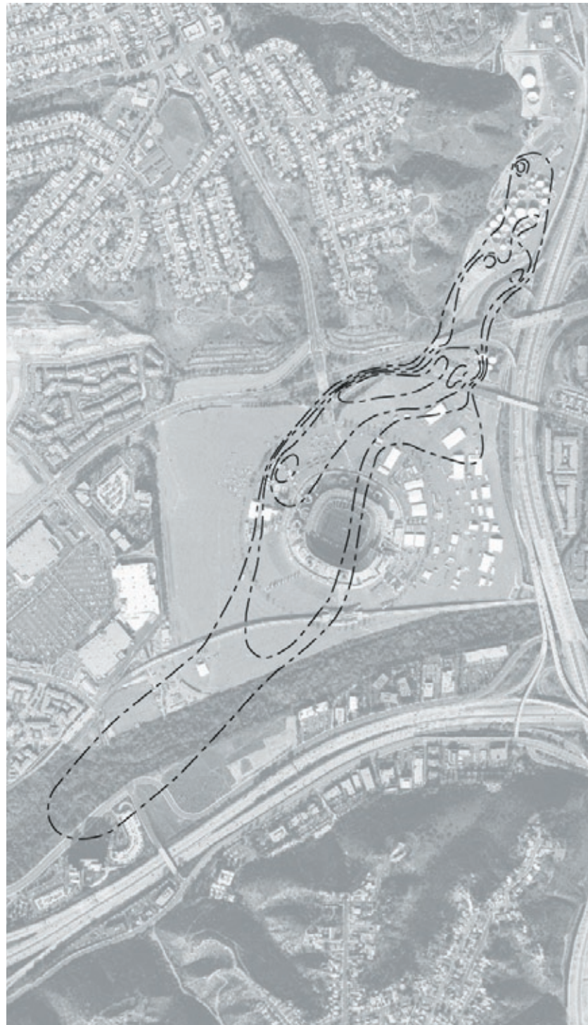
MTBE Isocentration Contours Source: Levine Fricke - Mission Valley Terminal Project No. 002-10143-02 MTBE Isoconcentration Map and Well Section (A-A') August 2003 Figure No. 9
