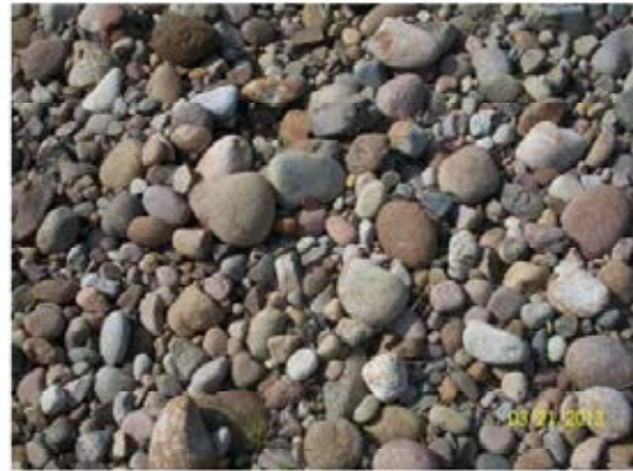
52. Reach 3 – A close up view of the pebble/cobble rock size that has been deposited on the channel bed. A one-cent coin, in the middle of the photo, provides a reference object in relation to the rock size.
