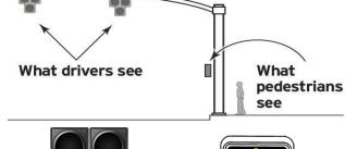
The Pedestrian Hybrid Beacon signal is dark. Traffic is free to move until a pedestrian presses button to cross.
