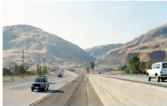
**Concrete barrier with paving to the base allows maintenance to mechanically sweep the shoulder.**
