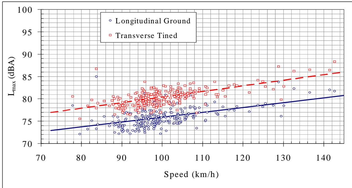
**FIGURE 1. Single Vehicle Pass-by Noise Measurements for Automobiles**
