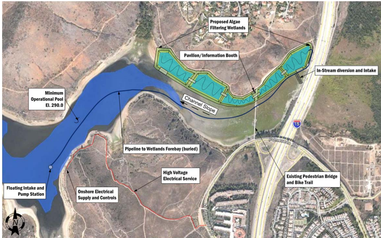
Figure 4-10. Conceptual Design Layout of Wetlands
