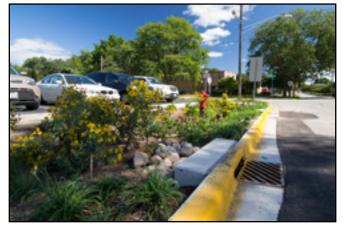
Filtering runoff with plant material
