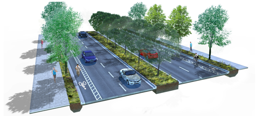
Linear gateway enhancements on Rosecrans Street north of Sports Arena Boulevard will include parkway bioswales with street trees, an urban path, bike lanes, and a planted median.
